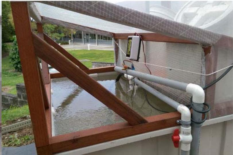
The solar system utilizes two 12v, 50 watt panels, mounted at a 90 degree angle to each other, and oriented south. The panels are slightly over sized for the power required so that during overcast days, the system can still operate normally. The eastern rising sun to strikes the first panel at sufficient angle to
